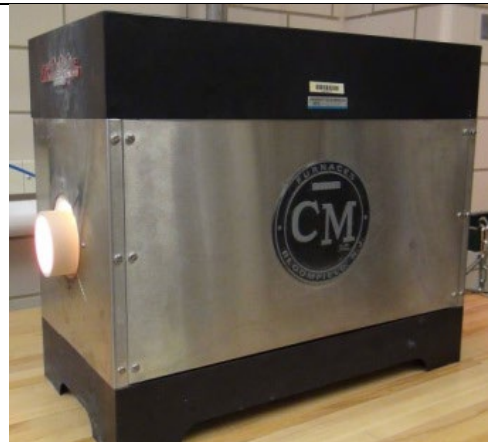
Figure 4: High Temperature tube furnace with an alumina furnace tube installed
