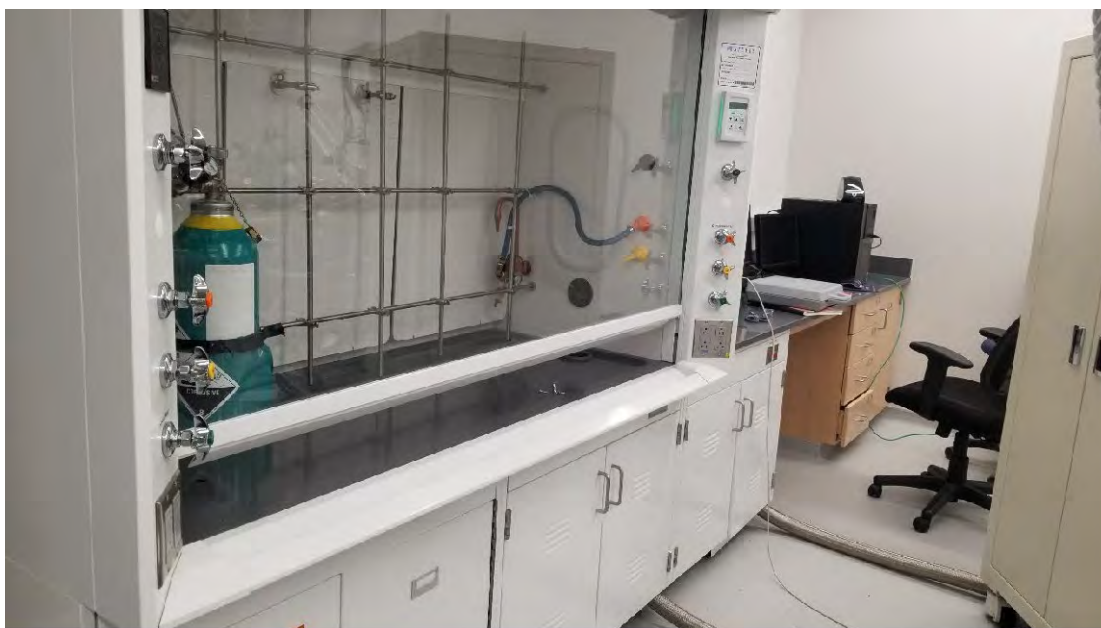
Figure 2 A proper example of a CFH when procedures are not underway.
