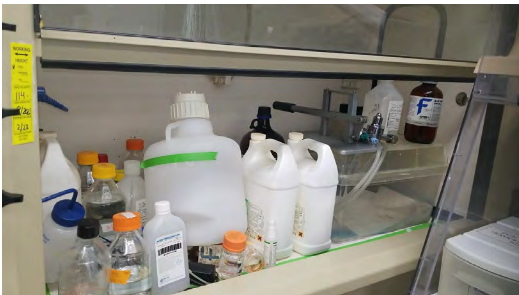
Figure 1 An example of a CFH improperly used for storage of containers. Overcrowding prevents proper airflow and containment.
