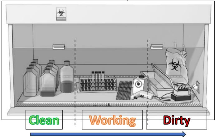
A typical layout for working from the clean to the dirty side within a Class II BSC. Clean cultures (left) can be inoculated (center); contaminated pipettes can be discarded and other contaminated materials placed in the biohazard bag (right). Reverse this arrangement for left-handed persons.
