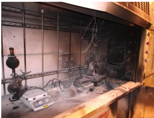
Figure 2. Damage to hood following BLEVE event.
