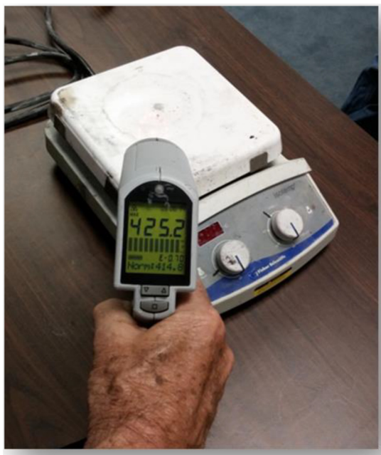
Figure 1. Infrared thermometer indicating elevated temperature on surface of hot plate while heating controls are in “OFF” position.
